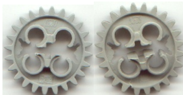
Broken old-style 24t gears (note that this style gear effectively had 3 axle holes)
